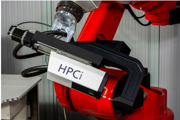
Joining tool (HPCi®) for robot thermal direct joining. © Fraunhofer IWS Dresden
